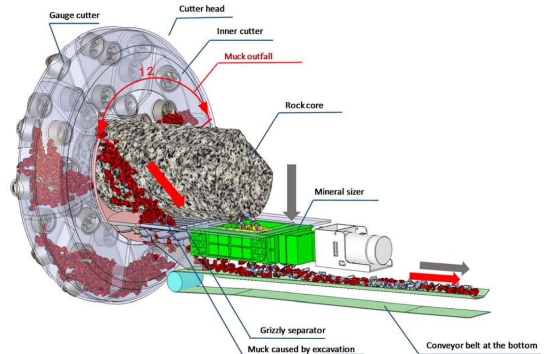
Ratio of a donut hole to a cutter head shall be set based on the geological conditions in which the machine is used, to make sure that construction machines are able to pass through the hole and that a rock core fragmentation must not be a critical operation in a whole process of excavation.
